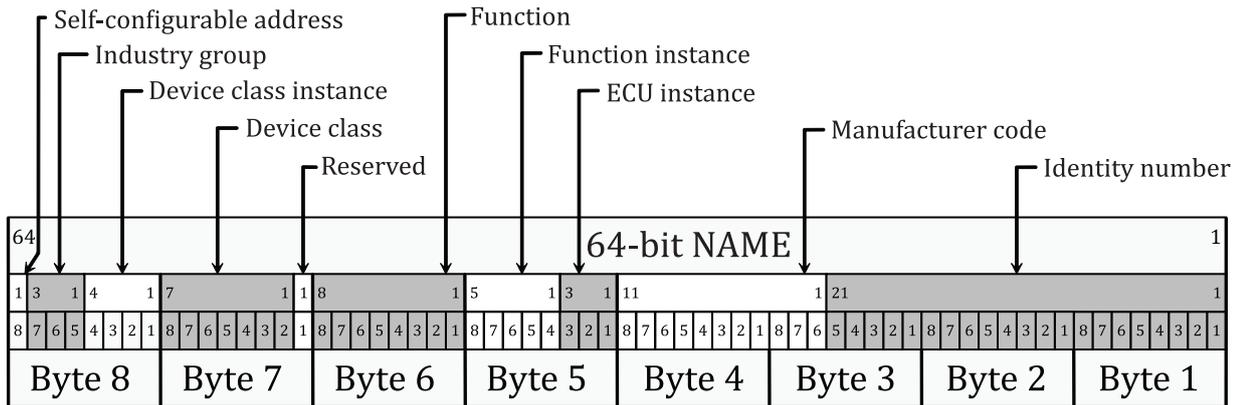
Figure 1 — Structure of the 64-bit NAME
