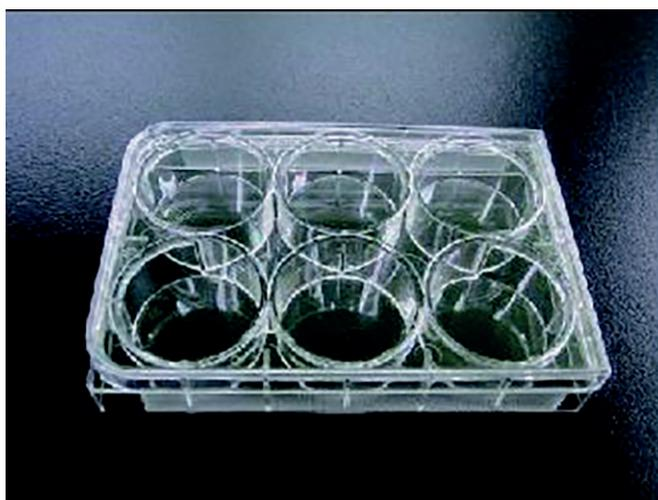
**Figure 2 — 6 wells plastic plate for plaque assay**
