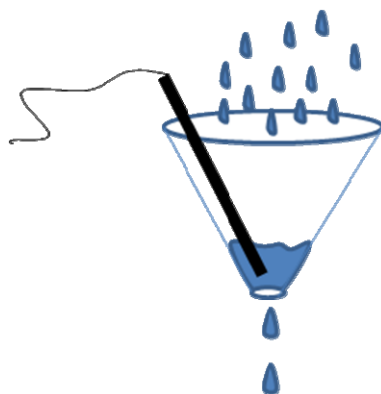
Figure 3 – An example of the positioning of the temperature sensor in a collecting vessel with a small outlet hole
