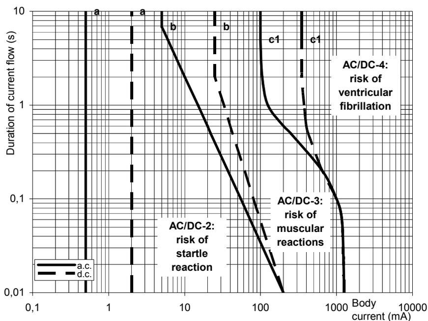
NOTE The "c<sub>1</sub>" curve is modified according to Table 12 of IEC/TS 60479-1; see also last paragraph of 4.1 of that standard.
