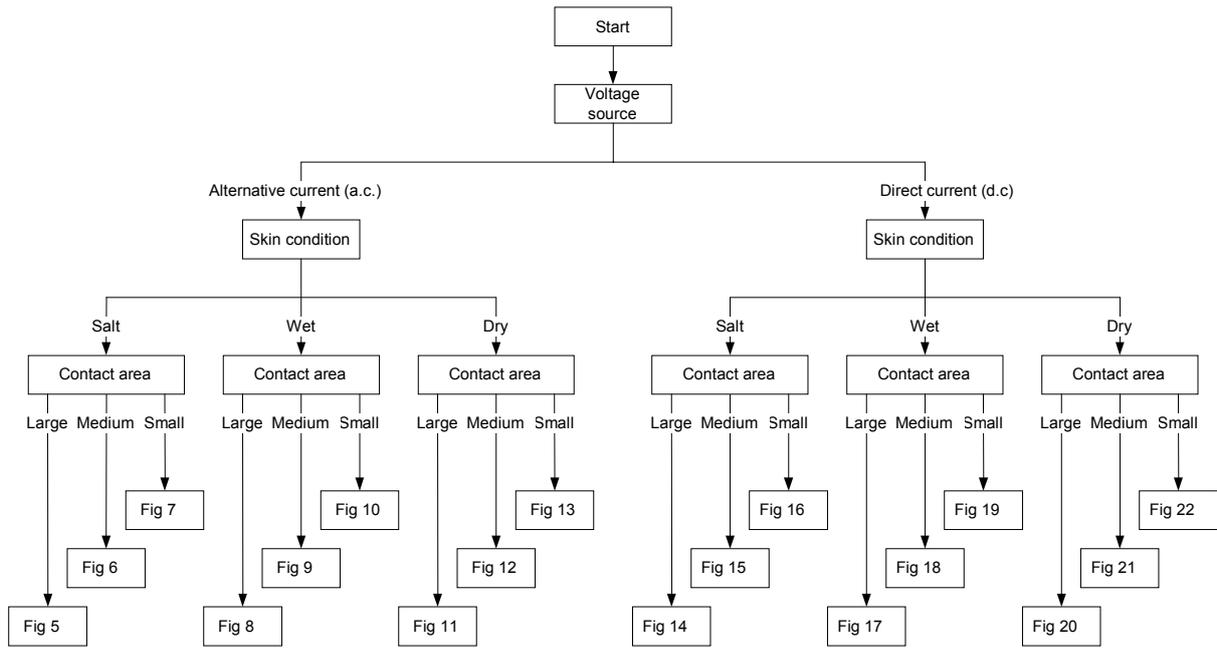
**Figure 4 – Flow chart to be used for the selection of the appropriate figure providing the maximum duration for each touch voltage threshold**
