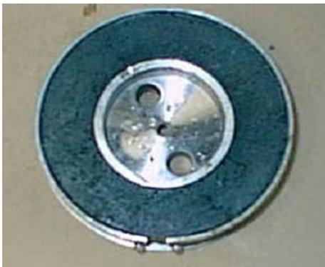
Figure 1 — Typical mould assembly (top view)
