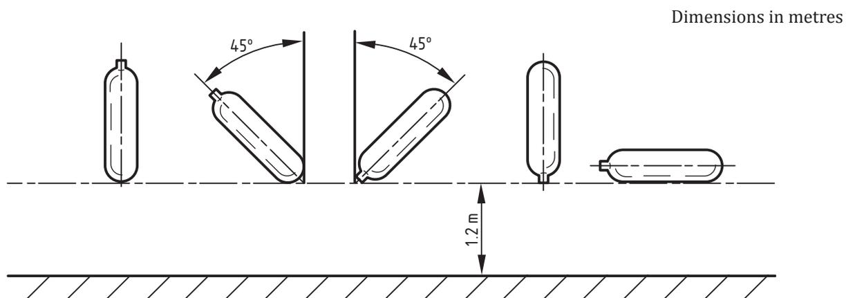
Figure 2 — Drop test
